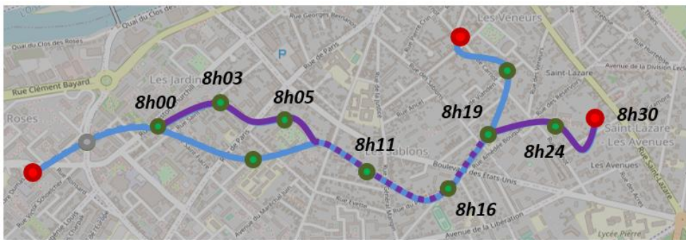
Figure 4.1-2 Scheme of a bus line with three terminals (in red), intermediate bus stops (in green), two routes (in blue and purple), and the time schedule of one trip on the purple route.
