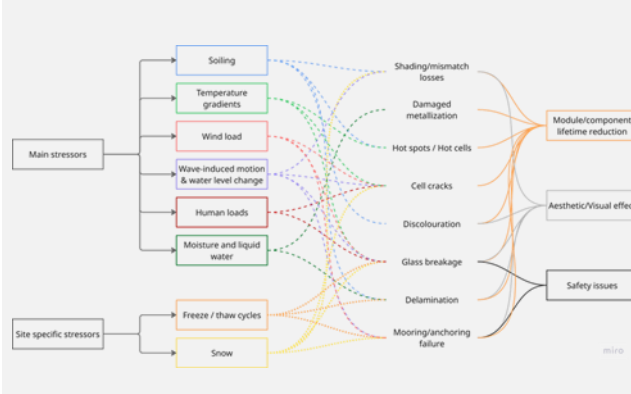
Stressors, induced degradation mechanisms and failure modes in FPV modules.
