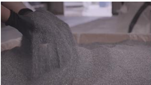
c) Silicon solar cell fragments after separation
