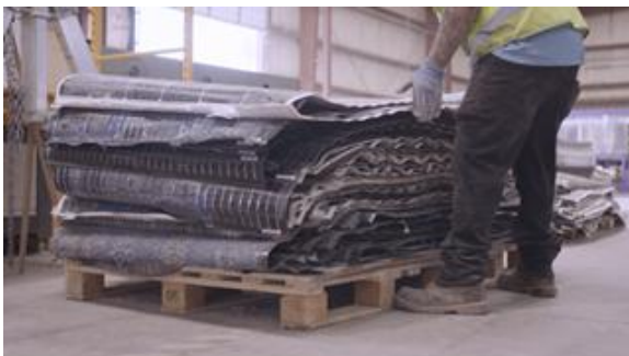
a) Laminate after glass removal
