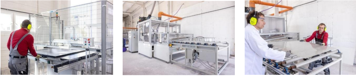
Figure 5. c-Si recycling process steps (from left to right): removal of junction box and frame, water jet cleaning unit, glass after water jet cleaning (Credit: PHOTORAMA – EU project ©European Union, 2025)
