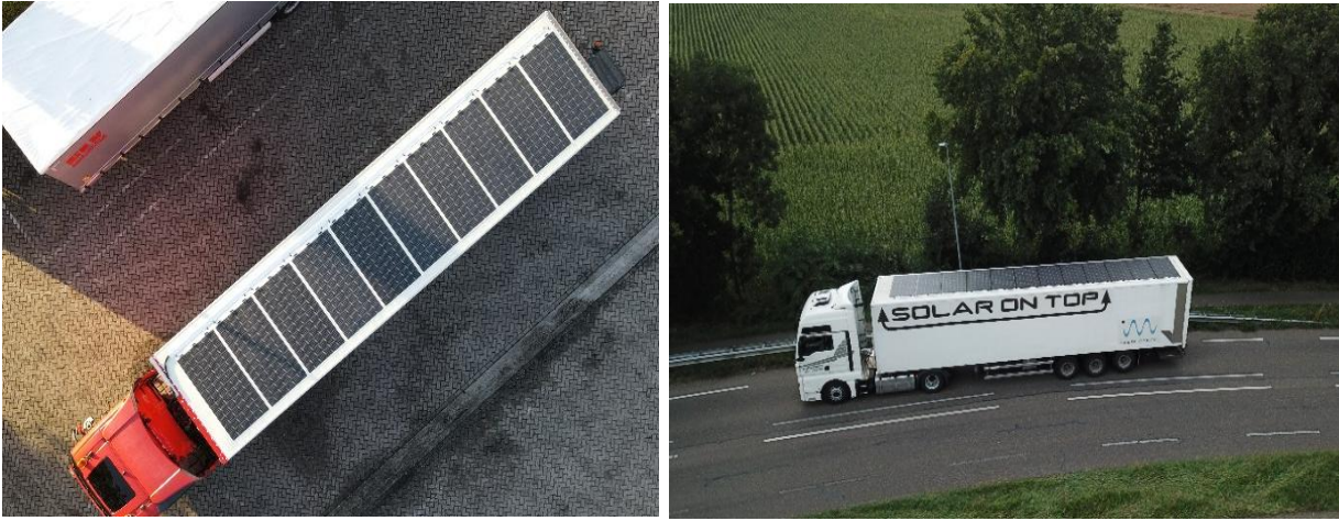
Fig. 7-1 Aerial view of SolaronTop showing comprehensive PV coverage on the truck-trailer roof surface
