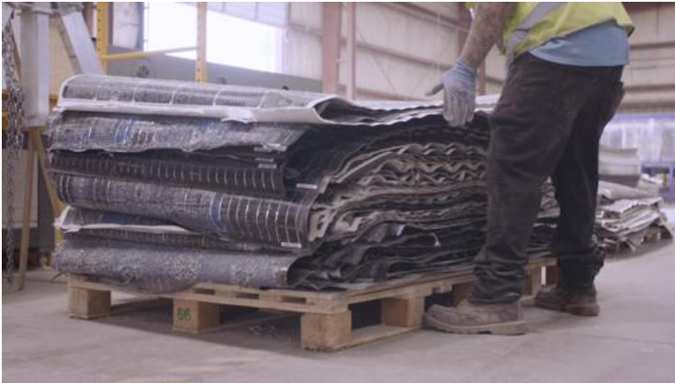
Laminate after glass removal
