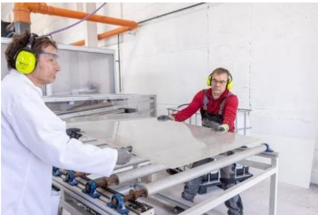
Glass after water jet cleaning
