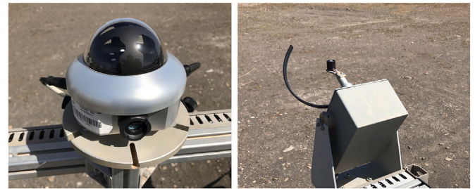
Fig. 3. Images of the SPN1 and RSP operated in Tabernas at CIEMAT's PSA.
