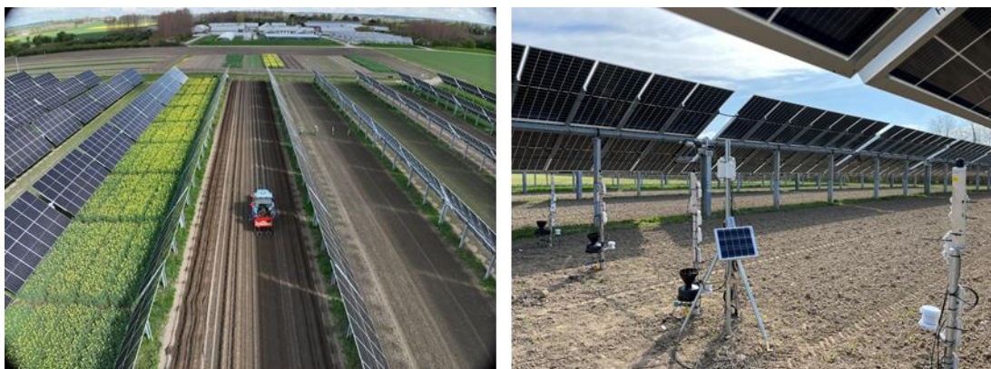
Figure 41: a) Example of agricultural work performed between rows with trackers facing opposite directions where work is taking place, and the remaining rows left in astronomical tracking mode. b) Four inter-row sensor masts for monitoring key indicators of agricultural productivity between rows in the test field. A fifth equivalent sensor mast is in the reference field. (Photo credit: Aarhus University, Department of Agroecology, and European Energy A/S)
