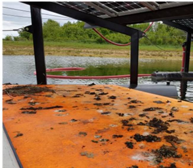
Figure 21. Biofouling and organic soiling observed on a reflective surface beneath a FPV system in [72].
